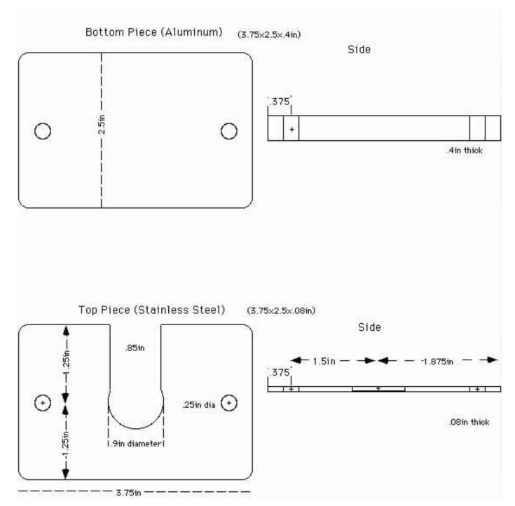
This clamps the electrochemical top (or any other glass fixture with an 18 mm o-ring joint) to the teflon etch cell
