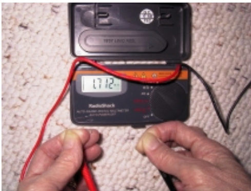
Measuring skin resistance with the multimeter
